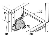
Attach cable with cable tie (32) to the motor carrier unit.
